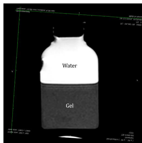
T2-weighted morphological MRI image of a bottle containing a PDMS / aqueous PVA mixture acquired with a Philips Ingenia 3T clinical MRI scanner
